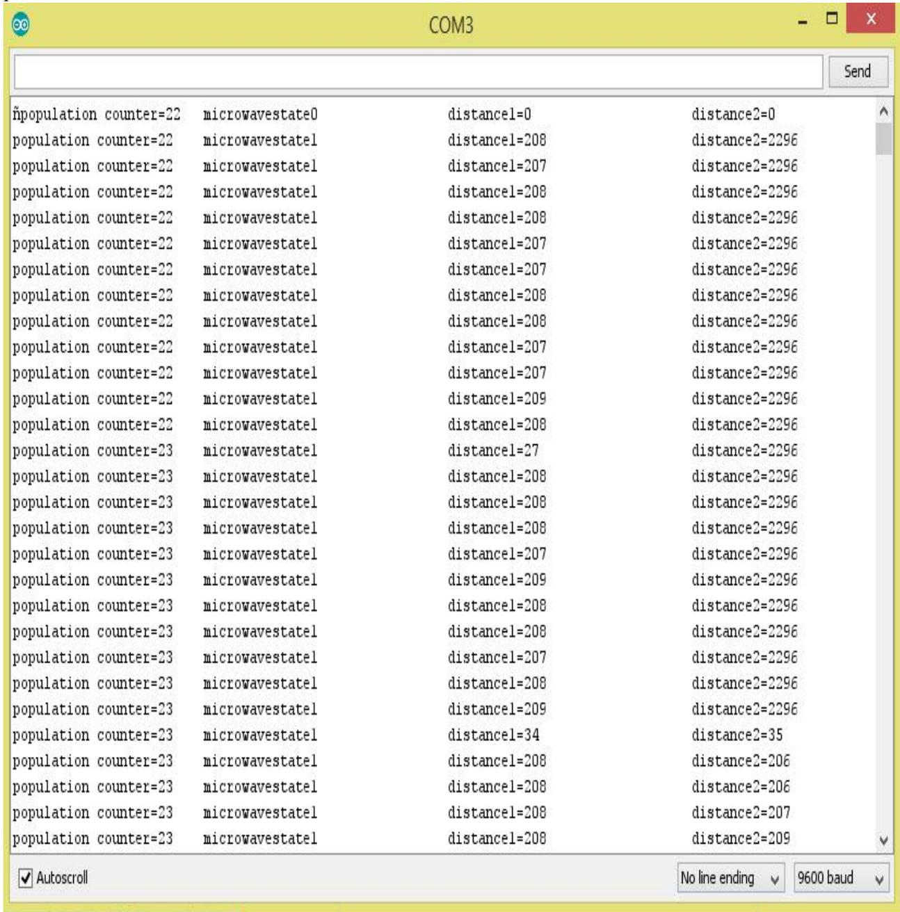
Fig 4: Serial Monitor Display of Population Counter, Microwave Sensor State and Ultrasonic Sensor1 and 2 Readings
