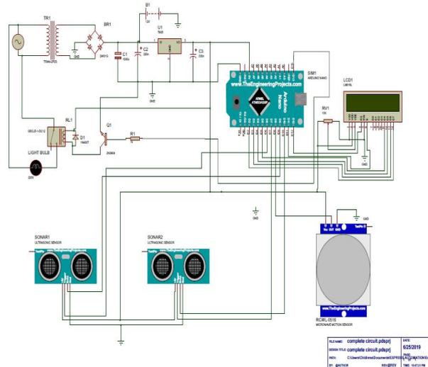
Fig 3: System Circuit Diagram.
