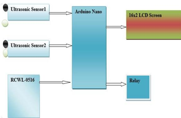
**Fig 1:** System Component Interaction.
