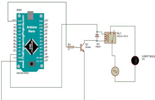
Fig 2: Relay switching Circuit.
