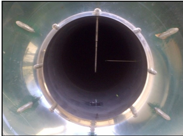
Figure 2: Wind tunnel intake
